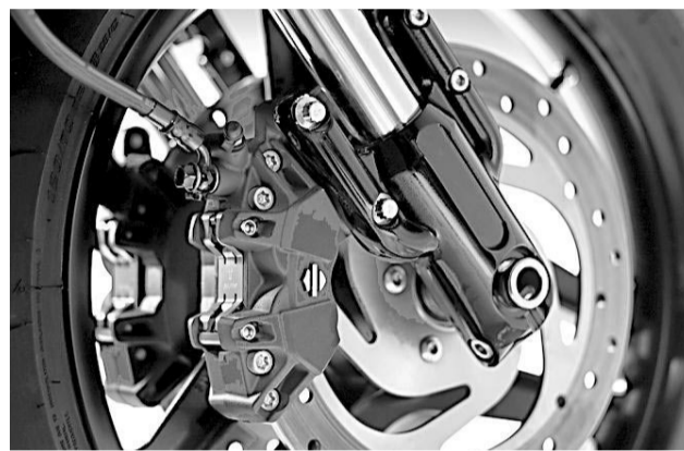
ROOTS Styling of the 2009 Harley-Davidson XR1200 is derived from the XR-750 dirt track racer. Racing influence is also seen in the simple instrumentation, above left. Four-piston Nissin calipers, above right, are used at the front.
