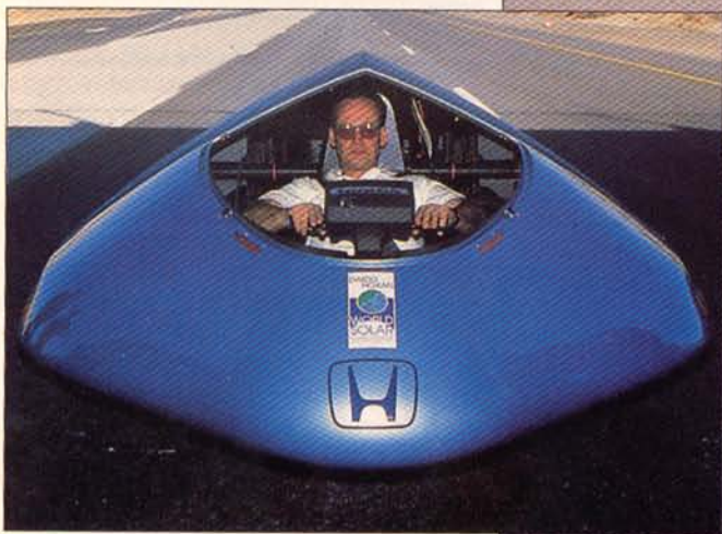
Tight fit: The driving position is reclining.
