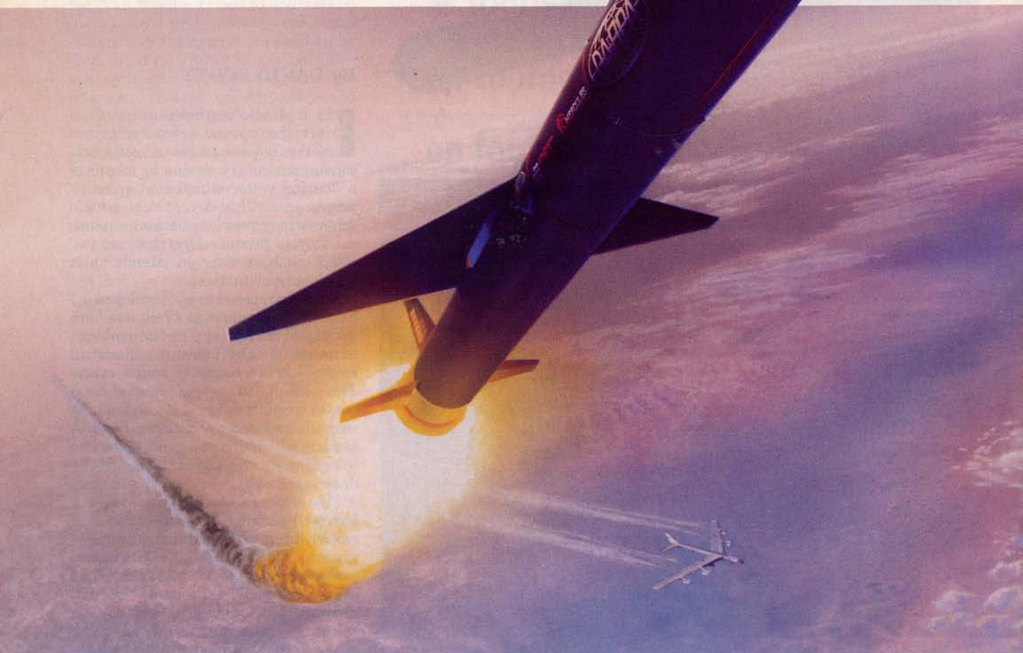
A Pegasus air-launched space booster climbs upward from the B-52 bomber that launched it.
