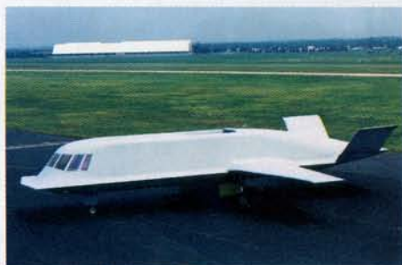
NORTHROP'S TACIT BLUE tested the compound contours that led to the B-2 in the '80s.
