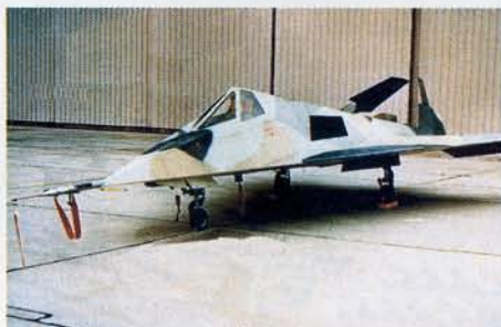
LOCKHEED'S EXPERIMENTAL HAVE BLUE proved the F-117A's faceted shape in the '70s.
