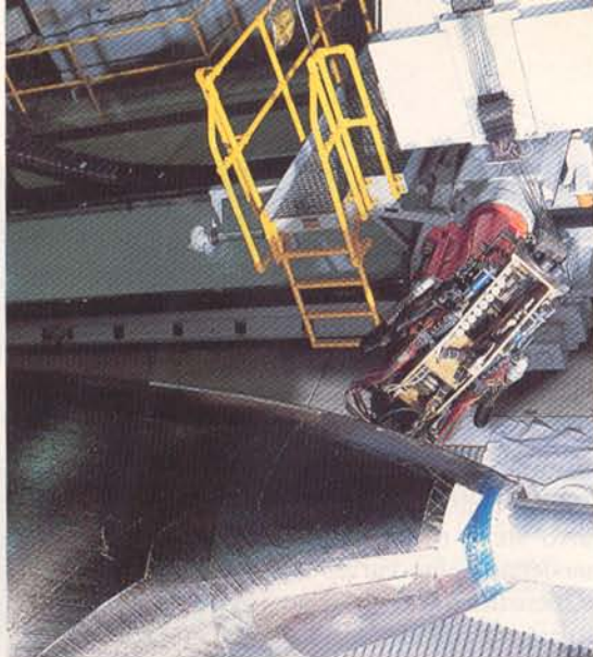
BUSINESS END: The head of a Cincinnati machine builds up a Horizon's nose.
