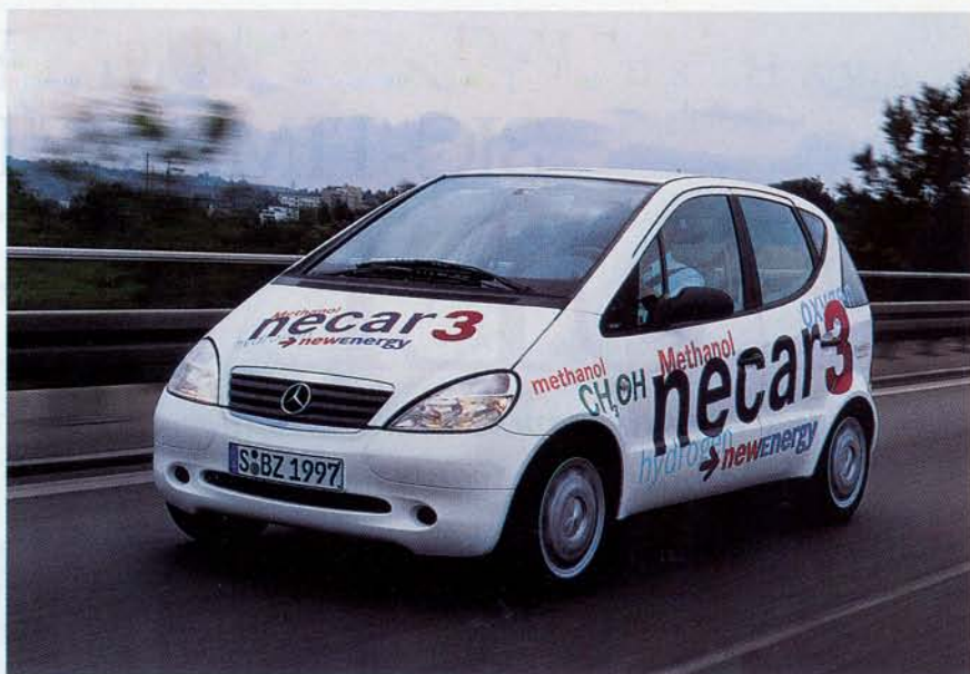
The latest Mercedes fuel-cell test car makes hydrogen onboard from methanol.
