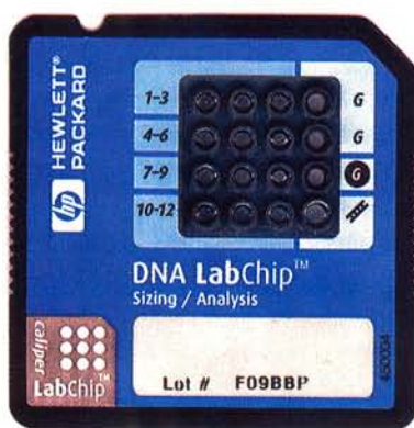
The top 12 “wells” in the LabChip used by Agilent Technologies (shown actual size in its housing at left) hold DNA fragments that get sorted by size as they flow through its channels. Other wells hold materials used in the sorting process.
