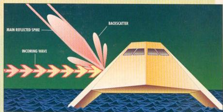
Specialized equations are used to predict the direction in which an incoming radar wave's reflected main spike and secondary backscatter will travel. A balanced stealth design angles the craft's surfaces to avoid any strong reflections back to the radar's source.
