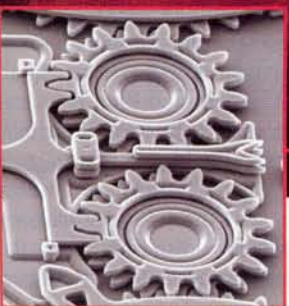
Safety lock The small photos show gears the size of a pollen grain (left) that spin in the prototype "stronglink" (center) developed by Sandia Laboratories for a nuclear bomb. The dozens of components, "grown" fully assembled, all fit on a tiny chip.
