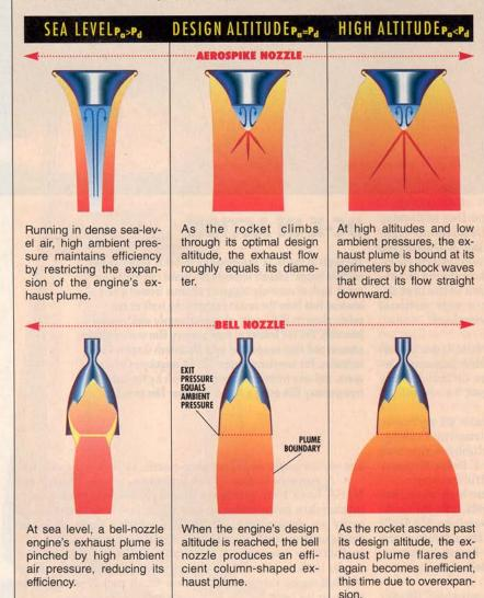
Pa=Ambient Pressure Pd=Design Pressure
