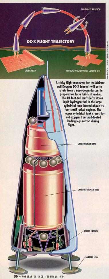
lasting off from the shimmering gypsum flats of the Army's White Sands Missile Range in New Mexico last September, the McDonnell Douglas Delta Clipper Experimental rocket, or DC-X, rose skyward to an altitude of 300 feet, then slowed to a startling, motionless mid-air hover—as if it were a helicopter. Tilting slightly, the craft next flew sideways for 350 feet. Fi-
