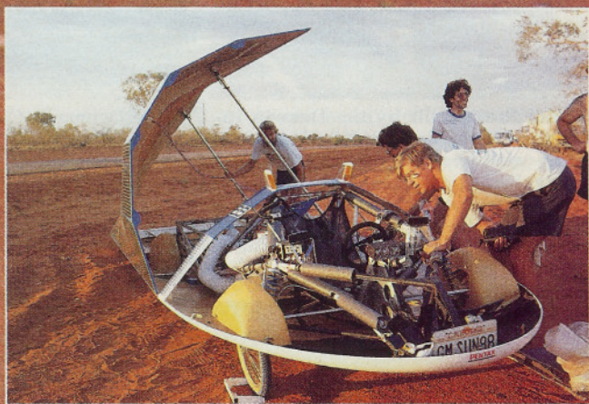
GM's Sunraycer (left) glides quietly through the outback. Car's approximate drag coefficient is an ultra-low 0.13. Strakes above cockpit and fins under tail aid stability in crosswinds. After a day's racing (above), team members monitor battery-charging rate and scold onlookers who let their shadows fall on the high-efficiency gallium-arsenide solar array. The author (top) snuggles up to a 62-wheeled road train. These leviathans traverse Australia's remote and railroad-less Northern Territory region, generating ferocious air turbulence.
