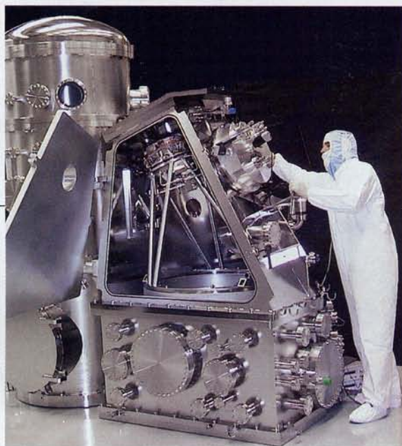
Sandia Labs' prototype prints chips using extreme-ultraviolet light.
