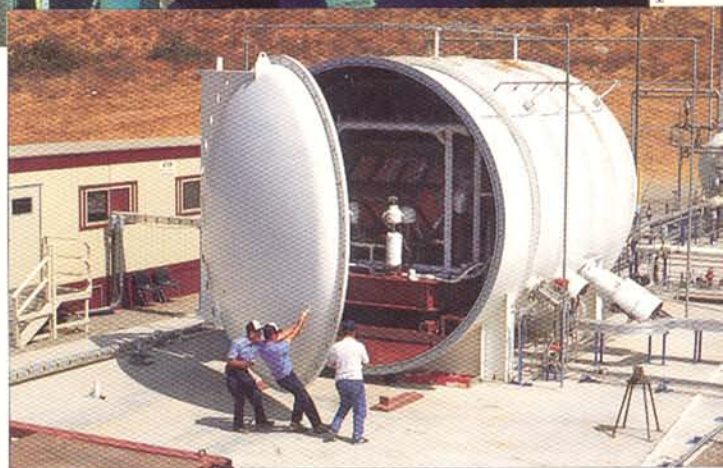
Technicians (above) at Wyle Laboratories in Norco, Calif., close an environmental chamber containing an 8-foot-long composite NASP fuselage and hydrogen-tank section. It is designed to withstand cryogenic (-420°F), thermal (1,300°F), and mechanical stresses that would be encountered in flight. Safe handling of hydrogen (right) is a must.
