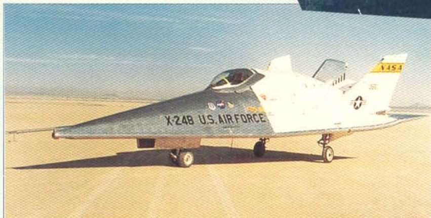
The X-15 (top) and X-24B rocket planes proved in the 1960s and 1970s that hypersonic flight and the wingless lifting body were workable ideas. Their shape and construction influence the X-30's design.
